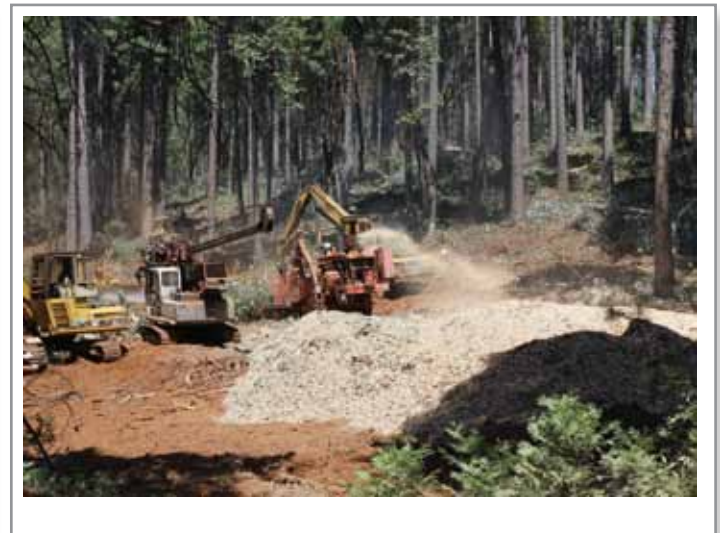
A wood chipper processes woody biomass from a restoration thinning project, Mt Hope Stewardship Project, Plumas National Forest.
